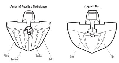
The best way to locate turbulence-free water is to view the transom while the boat is moving. This
